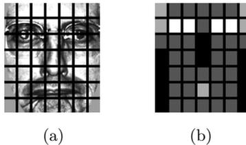
**Fig. 5.** (a) An example of a facial image divided into 7x7 windows. (b) The weights set for weighted  $\chi^2$  dissimilarity measure. Black squares indicate weight 0.0, dark grey 1.0, light grey 2.0 and white 4.0.
